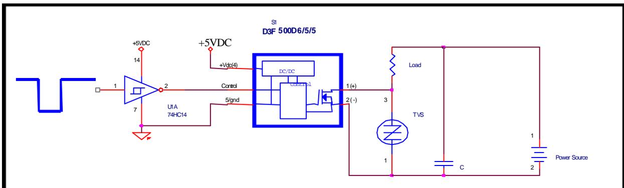
Figure 5 Switching Time Test Circuit
