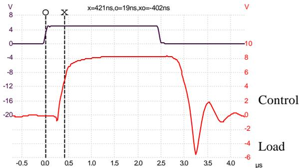
Figure 1 Turn-on delay is 402nS
