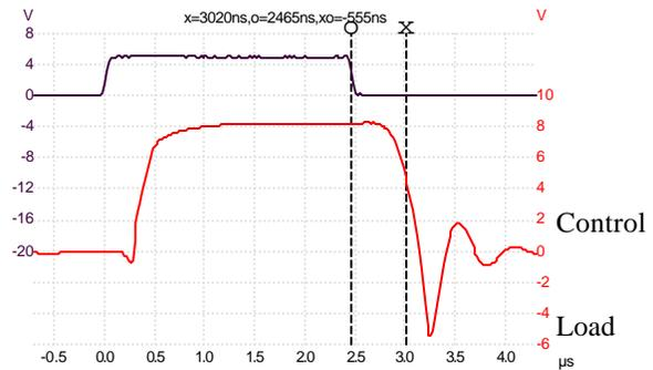
Figure 2 Turn-off delay is 555nS
